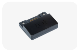
NFC Module ✓ NFC reader ✓ Pogo pin connection
